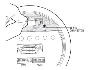
Figure 19. Installing the TXB-V into the ExSite
